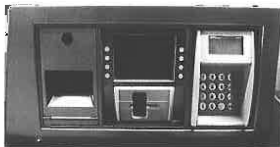
Picture 2: Terminal with GLOBALcom module
