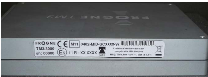
Figure 9: Placement of marking on the CPU. XX XX-yy is to be replaced by the approval number. 11 is to be replaced by the year of manufacturing.
