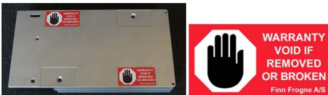
Figure 7 and 8: Factory sealing of the CPU unit and label for the factory sealing
