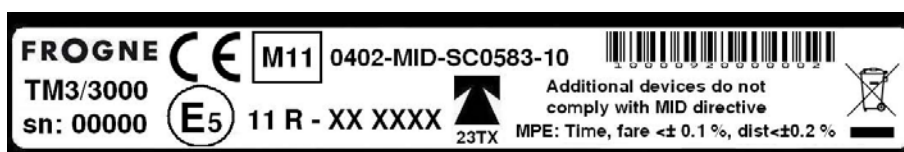
Figure 10: Layout of marking on the CPU
