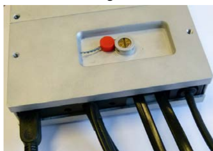
Figure 5: Sealing of lid to service area of CPU
