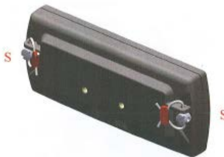
Figure 7: Sealing of display
