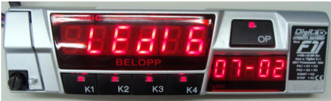
Figure 2: Central Processor Unit (CPU) with display, Digitax F1+
