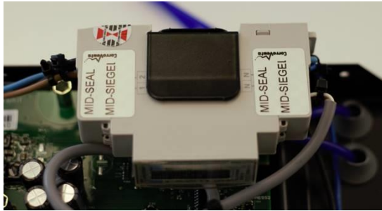
Figure 4. Placement of CEMP seals, on terminal cover of meter and the display case
