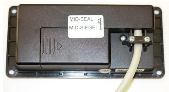
Figure 4. Placement of CEMP seals, on terminal cover of meter and the display case
