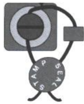
Figure 4: Figurer of the taximeter F1+ (CPU and display) with the lid and the physical sealing.
