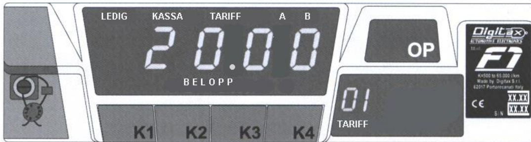
Figure 3: Figurer of the taximeter F1+ (CPU and display) with the lid (removed from the taximeter) for sealing the power supply, printer and communication cable, and also the connection for the black key.
