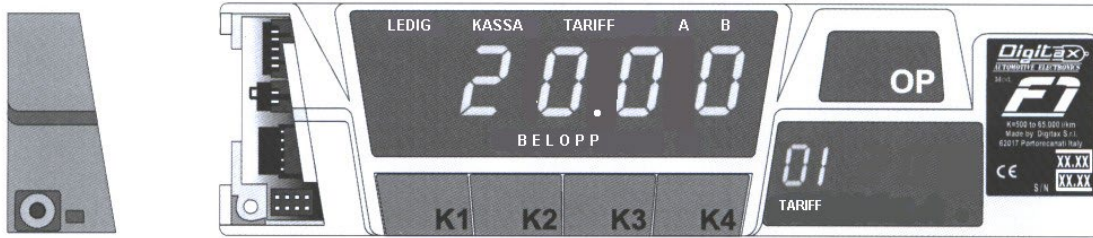
Figure 3: Figurer of the taximeter F1+ (CPU and display) with the lid (removed from the taximeter) for sealing the power supply, printer and communication cable, and also the connection for the black key.
