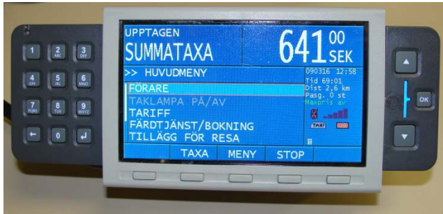
Picture 2: Central Processor Unit with display MTME350
