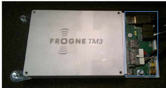
Figure 4: How to fasten the CPU
