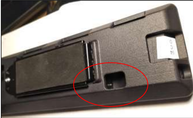
Figure 18: Sealing of display TT430 in RM1c casing, marked with a read ring
