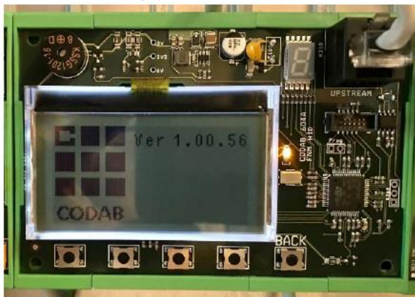
FuelNet display module connected (temporarily) to FuelNet Manager
