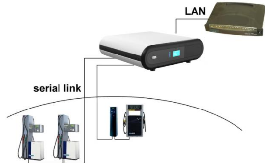
Figure 3: Typical configuration for Fusion forecourt system with embedded GUI for unmanned stations
