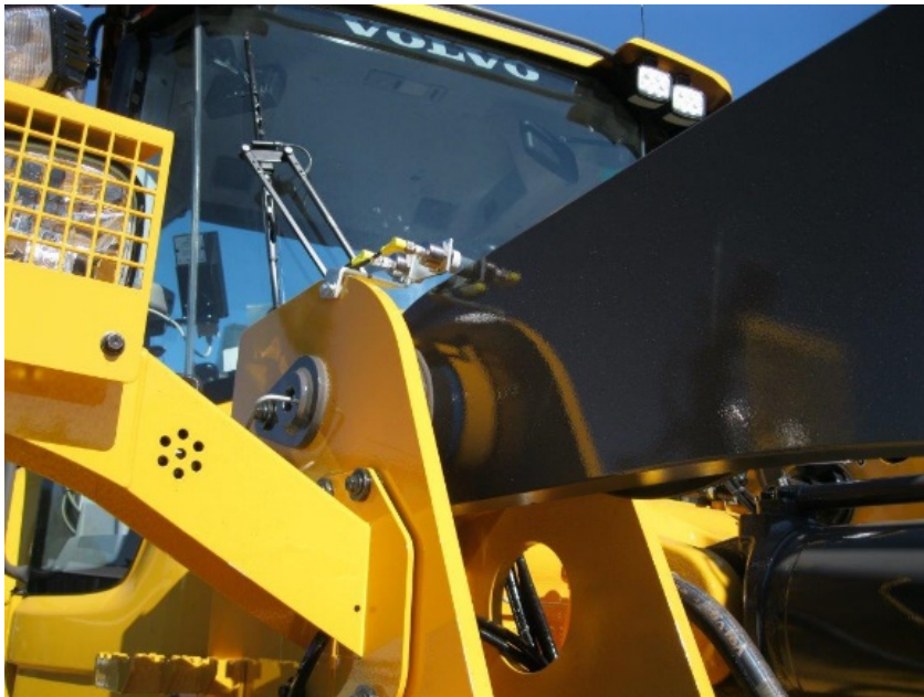
Picture 3. Mounted inductive sensors for start and stop of dynamic measurement.
