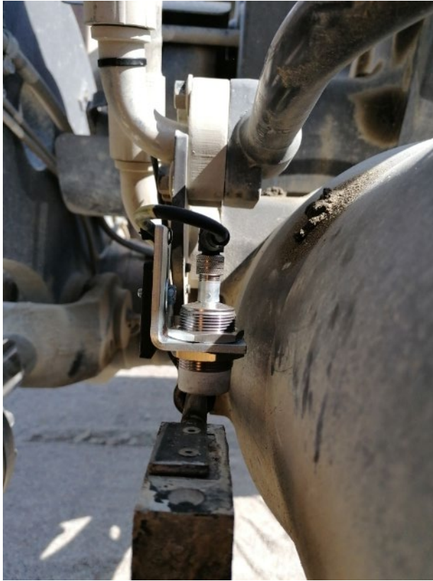
Picture 4. Mounted tilt limiting device.
