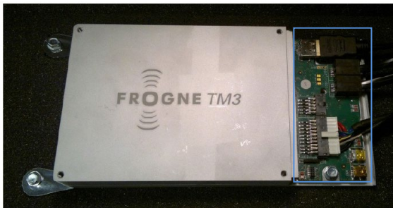
Figure 4: How to fasten the CPU
