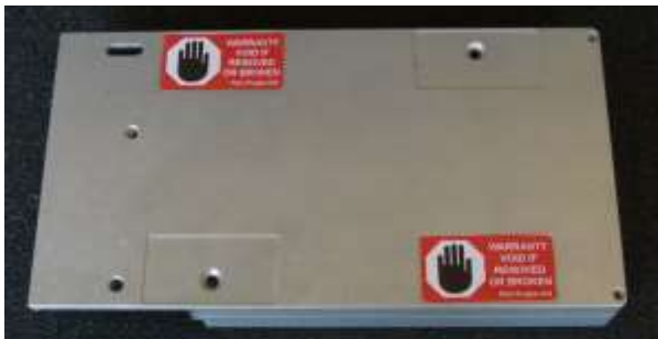
Figure 7 and 8: Factory sealing of the CPU unit and label for the factory sealing
