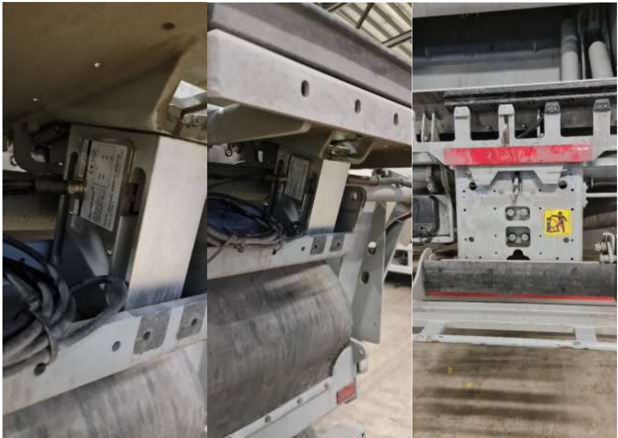
Figure 5. The weighing instrument (Installed Behind the Load Receiver Frame)
