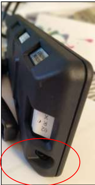
Figure 19: Sealing of display TT430 in RM1r casing, marked with a read ring
