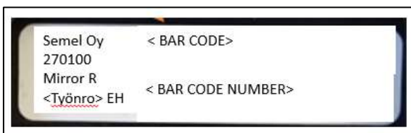
Figure 30: Example of label sticker for display TT430 in casing RM1r.
