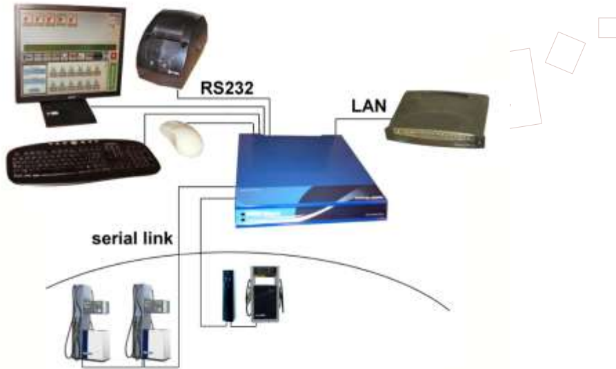
Figure 1: Typical configuration for Fusion forecourt system with embedded POS
